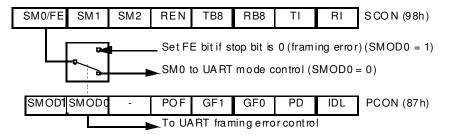
When this feature is enabled, the receiver checks each incoming data frame for a valid stop bit. An invalid stop bit may result from noise on the serial lines or from simultaneous transmission by two CPUs. If a valid stop bit is not found, the Framing Error bit (FE) in SCON register (see Table 11-4) bit is set.
