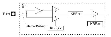
Figure 13-2. Keyboard Input Circuitry
