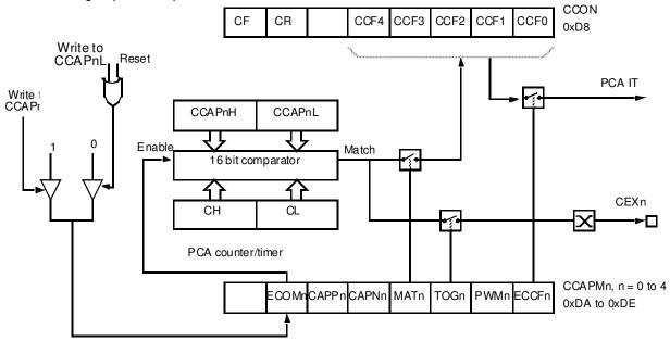
Before enabling ECOM bit, CCAPnL and CCAPnH should be set with a non zero value, otherwise an unwanted match could occur.
