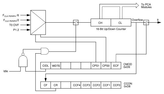
**Table 10-1.** CMOD Register CMOD - PCA Counter Mode Register (D9h)
