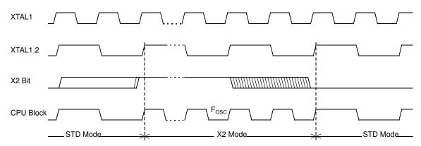
The X2 bit in the CKCON0 register (see Table 6-1) allows to switch from 12 clock periods per instruction to 6 clock periods and vice versa. At reset, the speed is set according to X2 bit of Hardware Config Byte (HCB). By default, Standard mode is activated. Setting the X2 bit activates the X2 feature (X2 mode).
