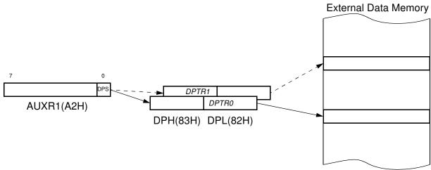
**Table 7-1.** AUXR1 Register AUXR1- Auxiliary Register 1(0A2h)
